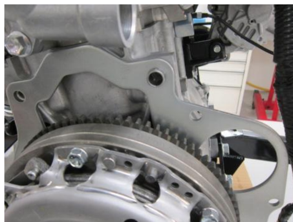
Figure 36: Gearbox spacer and dowels
