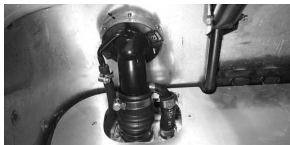
Figure 145: Filler cover and boot carpet removed
