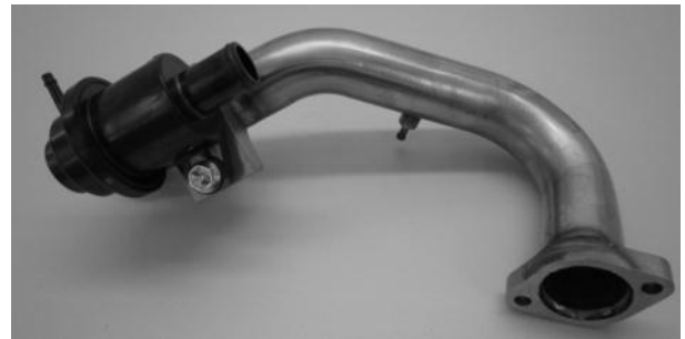
Figure 41: Compressor outlet pipe
