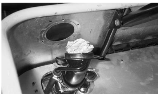
Figure 147: Old filler boss removed
