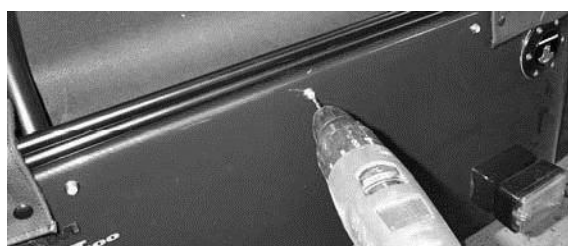
Figure 154: Drilling central popper on SV
