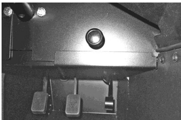
Figure 55: Heater control location
